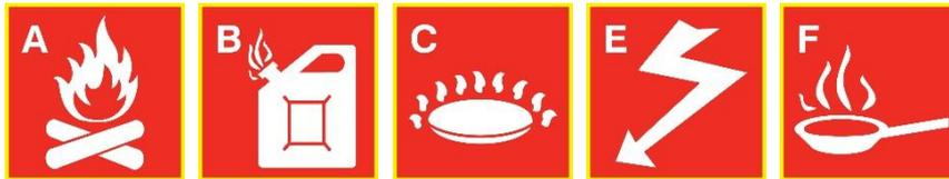
**The SPITA Firefighter is not suitable for extinguishing burning coal. Tested for electrical equipment fires up to 100kV and suitable up to 1000V.**
